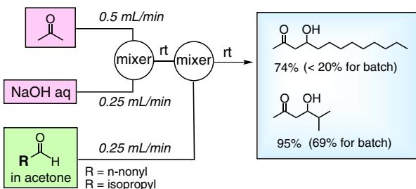
Efficient aldol condensation of acetone was achieved in a biphasic system by using the microfluidic apparatus.
